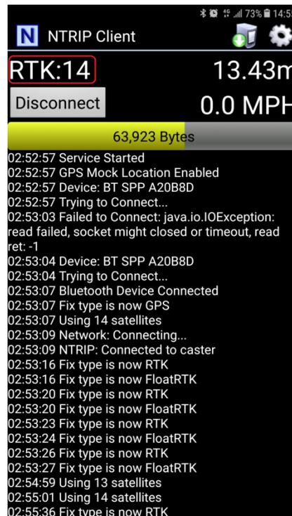
10. When surveying a group of locations within walking distance, can leave S100 powered up, taking the range pole or tripod to next location to survey. Switch to the Lefebure NTRIP Client App to check if S100 is in RTK Fix state before recording the next location position with Data Collector App. The setup procedure only needs to be performed once. Later use only need to run Lefebure NTRIP Client and connect.
